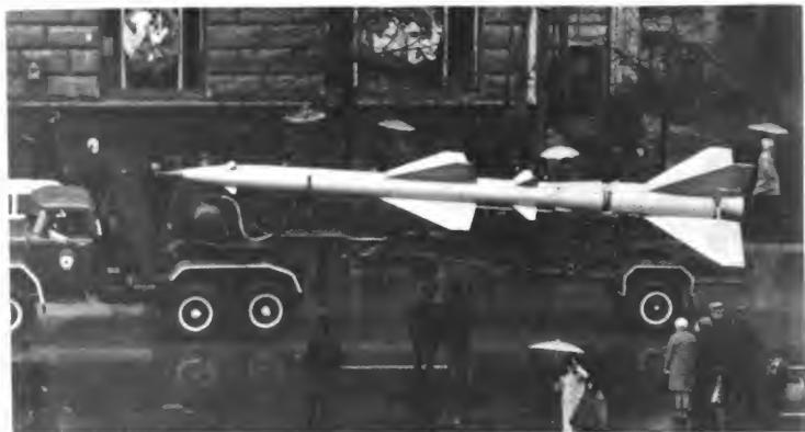
Figure 6-40. SA-2 GUIDELINE. A medium-range surface-to-air missile transported on a truck-towed trailer/launcher. The main SAM system in the Soviet Air Defense Forces (PVO Strany), GUIDELINE is also deployed with Soviet Ground Forces in Europe and has been exported to satellite nations.
